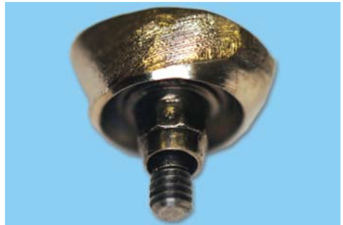
4 Intaglio surface of custom abutment coping after casting.
